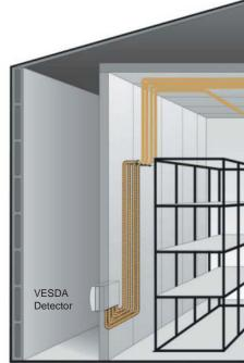
Figure 3. VESDA detector located externally to the protected area
